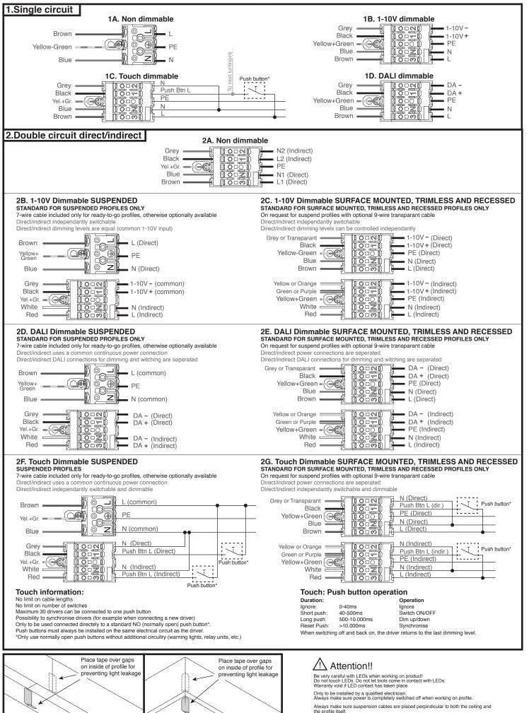
When connecting multiple parts of a structure always make sure LED polarity is respected. This means connecting white to white and grey to grey wires.
